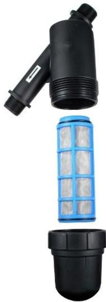
The Y Hose Filter is used with Drip Irrigation and is installed between the hose vacuum breaker and the pressure regulator. It helps to protect drip emitters, drippers and soaker hose drip line from rust, sand and other impurities that may clog them. It has a 3/4" female hose swivel inlet and a 3/4" male hose thread outlet.
