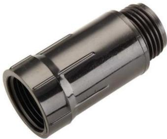
A pressure regulator reduces household water pressure to a set pressure for use with a drip tape system. **Always install a pressure regulator after a valve and filter.** They are not designed to be operated under constant pressure - The regulator only reduces pressure under flow.
